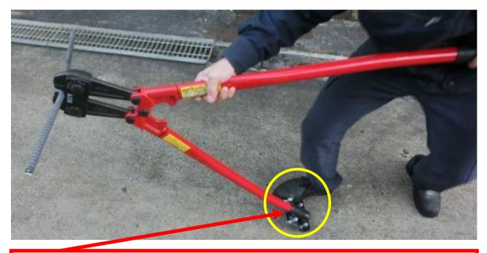
Placing the under handle with the BC STAND on the ground can change the force direction.
