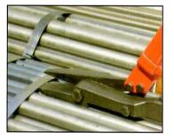
In this situation, it's difficult to insert the blade between steel strap and metal pipes.
