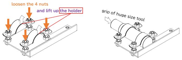
First, loosen the 4 nuts on the holder then lift the holder up and put the grip of huge size tool from HIT into the holder.
