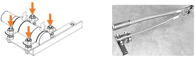
Next push down the holder and fasten nuts until the tool won't move around.
