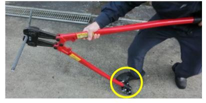
Place BC STAND with the handle on the ground and step on it. This can sure the operating will be stable, also change the direction of force when cutting materials.
